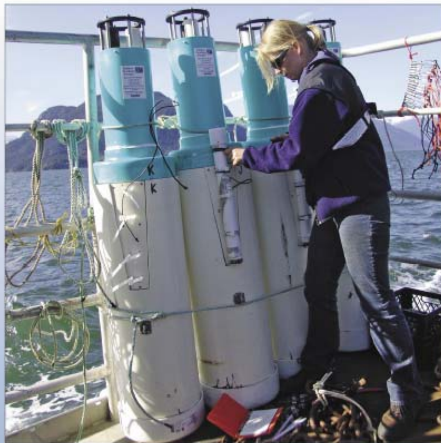
Heidi Lydersen prepares VR-3 units for deployment as part of the test trials preceding the construction of the permanent array.
